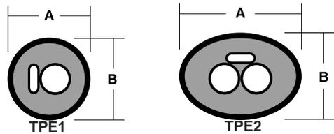
TPE1 - ONE 1/2" PROCESS LINE WITH LOW TEMPERATURE TRACER
